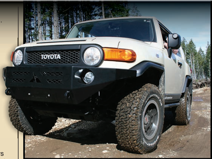
6061 T6 aluminum is used to construct the Aluminess bumper, with the main plating being 5/16-inch thick. The two recovery hooks are 1" thick by 3" deep—burly. You can order it with a basic brush guard, or as a full bull bar-type design. To see them all, go to http://aluminess.com/fj-cruisers.htm .
