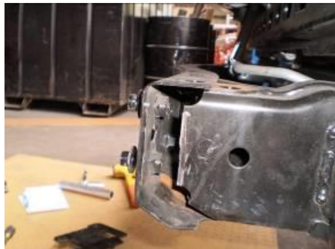
Figure 8b. Crossmember weld after cutting.
