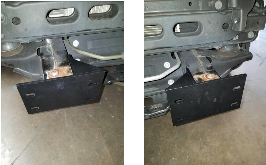
Figure 9. Steel angle brackets bolted to the passenger (left) and driver (right) frame horns.
