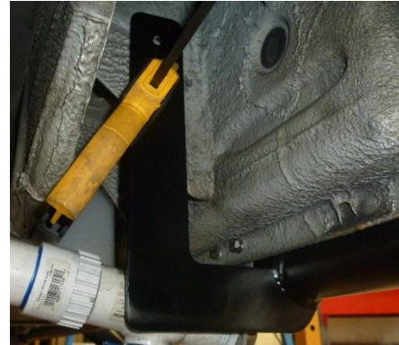
Figure 3: Rear Blade Against Body of Van
