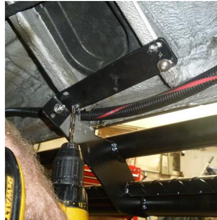
Figure 7: Center Mounting Bracket Against Front Body Brace.
