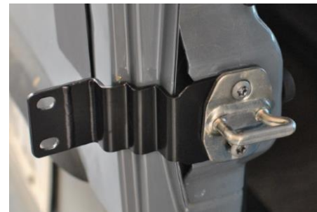
Figure 5: Driver's Inside Door Latch Bracket Installed
