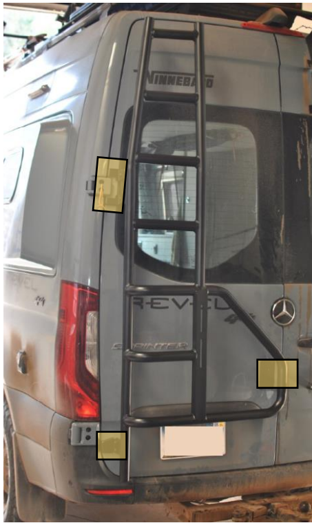
Figure 3: Protective Tape Locations on Door
