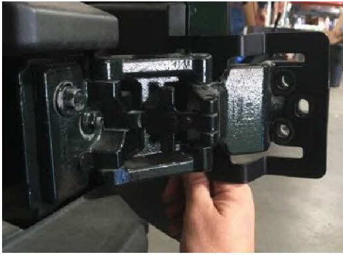
Figure 3: Bracket Installed Over Factory Hinge
