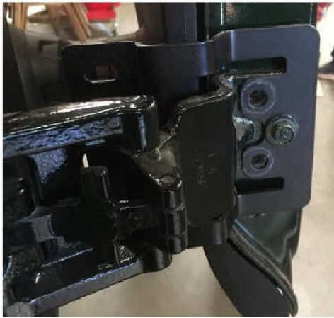
Figure 4: Hinge Placed Back into Position
