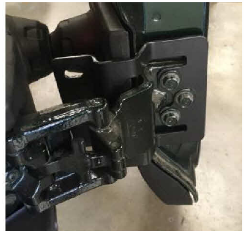
Figure 6: Inside View of Installed Lower Hinge Bracket
