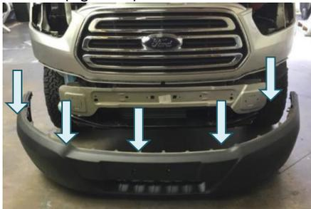
Figure 10: Front Bumper Removal
