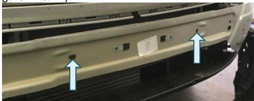
Figure 11: Holes to be Used for Installation
