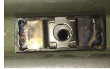
Figure 12: Attachment Bracket Holes Through Sub-Frame
