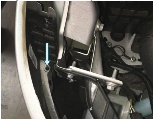
Figure 2: Bolts Underneath the Headlights
