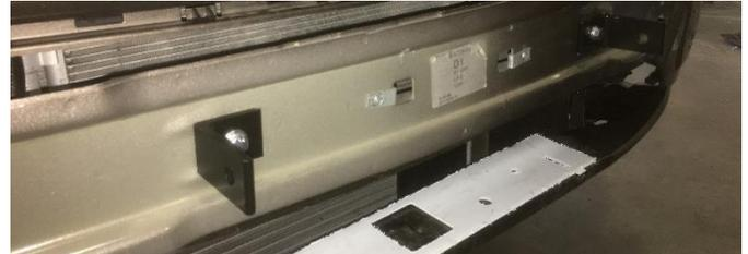
Figure 13: Attachment Brackets Attached to Sub-Frame
