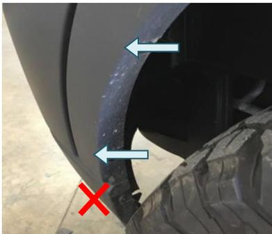
Figure 3: Fender Flare Plastic Rivets
