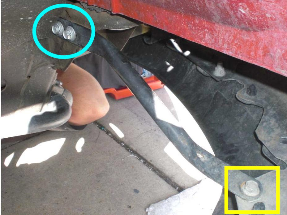
***Figure 1: Stock bumper tension rod***
