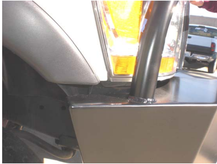
Figure 3: Correct body gap with new bumper installed
