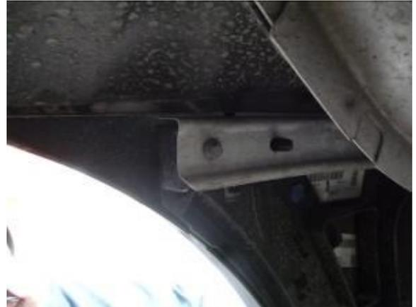
4. Unclip and remove the inner fender lining which will give you access to the fender flare clips.
