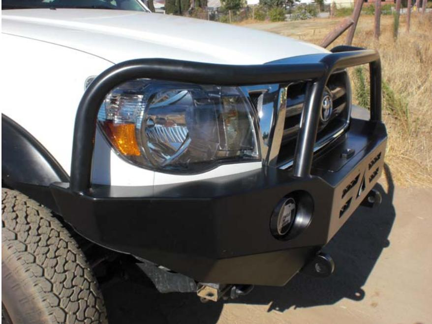
12. Visually inspect the bumper to make sure it is centered and level, then tighten down the nuts
