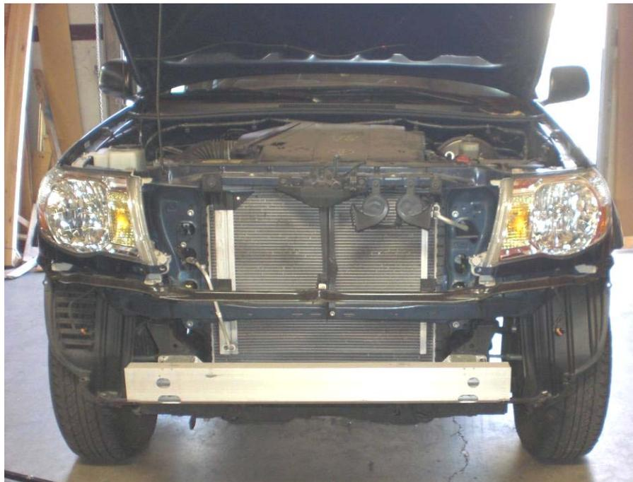
6. The aluminum beam in the center must be removed—there are three nuts on each side holding it on as seen in the picture below; unscrew these and slide the beam off. **NOTE: Do NOT throw these nuts away, you will be re-using them for your new Aluminess bumper**
