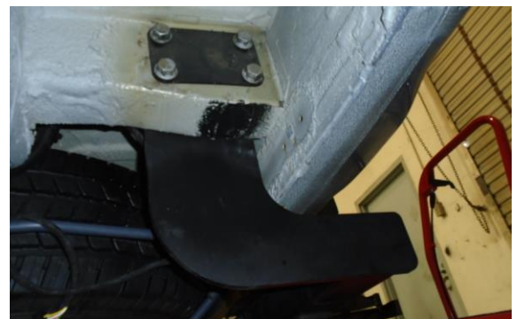
Figure 1: Four (4) of the Hitch Mounting Bolts
