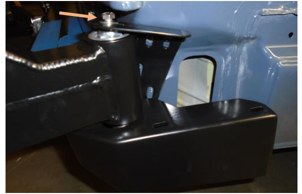
Figure 10: Pre-Mounting Axle Support Brackets
