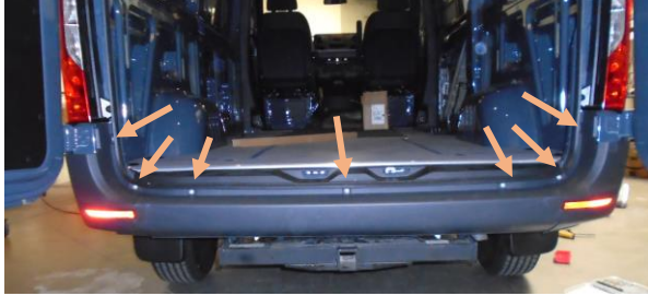
Figure 2: Torx Bolts on the Rear Bumper
