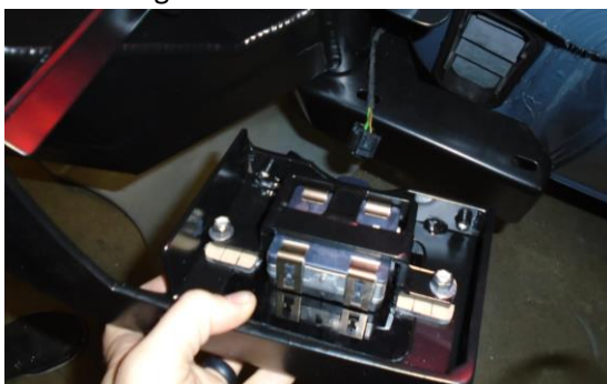
Figure 14: Blind Spot Sensor Installation
