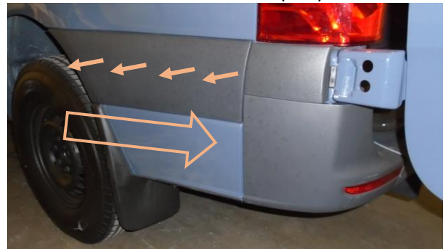
Figure 5: Side Panel Removal
