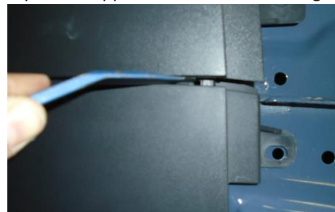
Figure 7: Removing Small Plastic Panel from Rear Bumper
