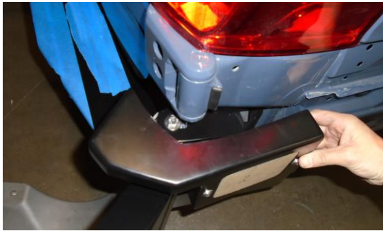
Figure 13: Installation of the Trim Assembly
