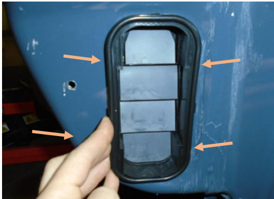
Figure 9: Air Pressure Relief Insert Removal
