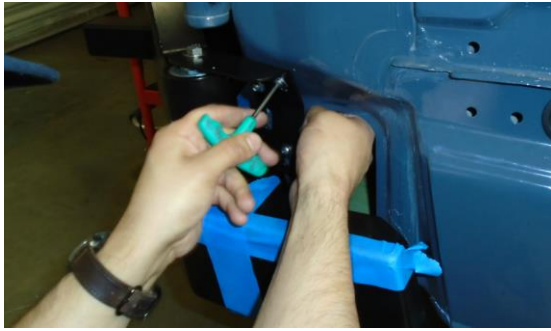
Figure 12: Tightening Hardware Through Insert Opening
