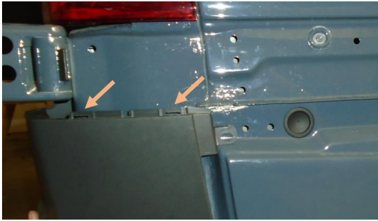
Figure 8: Small Plastic Panel Removed
