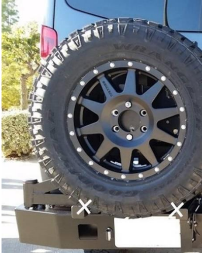
Figure 16: Tire Resting Correctly on Swing Arm
