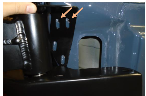
Figure 11: Drilling for Axle Support Bracket
