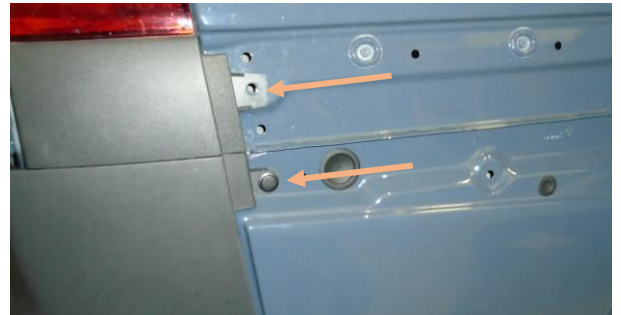
Figure 6: Plastic Rivets Underneath the Side Panel
