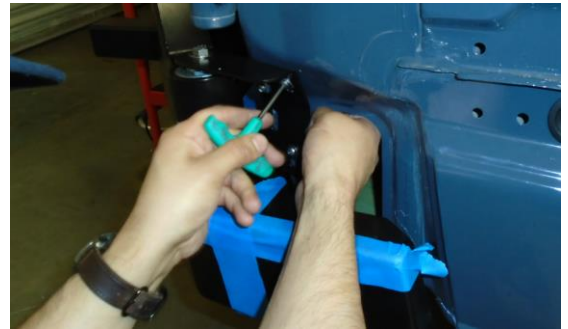
Figure 12: Tightening Hardware Through Insert Opening
