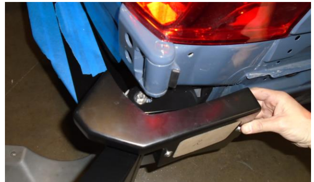
Figure 13: Installation of the Trim Assembly
