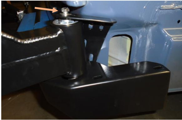
Figure 10: Pre-Mounting Axle Support Brackets
