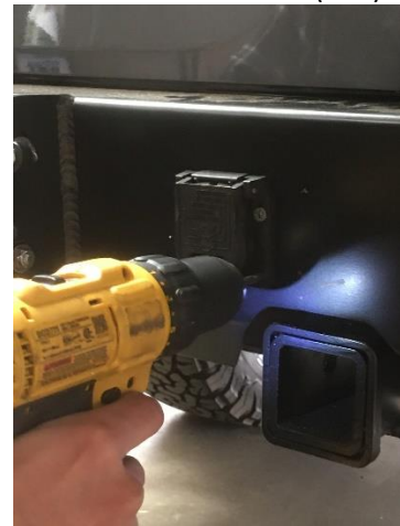
Figure 15: Installation of the trailer plug
