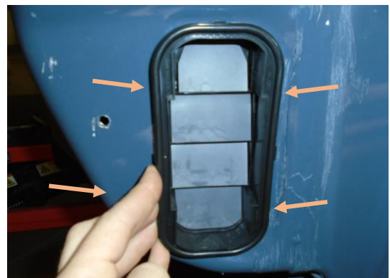
Figure 9: Air Pressure Relief Insert Removal
