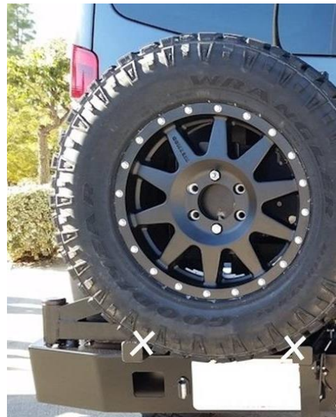
Figure 16: Tire Resting Correctly on Swing Arm
