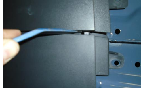
Figure 7: Removing Small Plastic Panel from Rear Bumper
