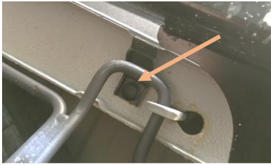
Figure 3: Plastic Rivets Underneath Bumper
