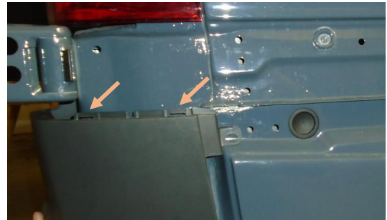
Figure 8: Small Plastic Panel Removed
