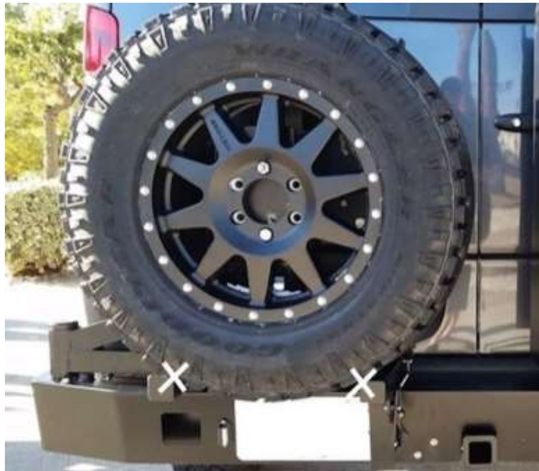
Figure 1. Rest tire on both support arms (before tightening the lugs or U-bolts down).
