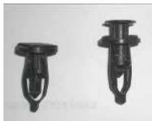
Figure 3: Toyota plastic fasteners, showing closed (left) and open (right) positions
