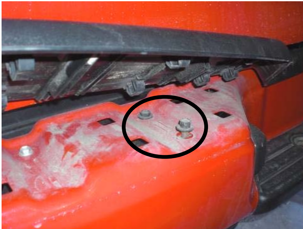
Figure 5: Stock plastic cover removed with mounting bolts exposed
