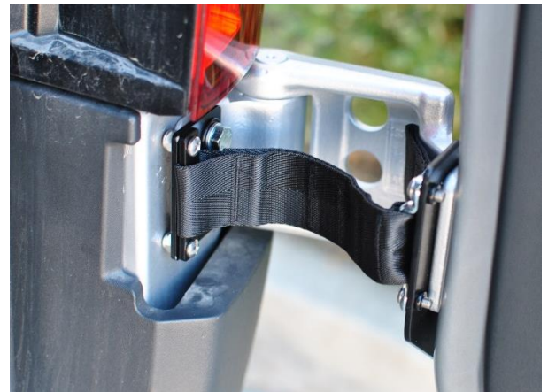
Figure 8: Door Limiting Strap Installed
