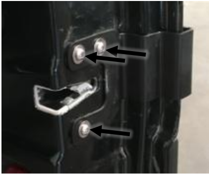
Figure 8: Installed Inner Passenger Door Bracket
