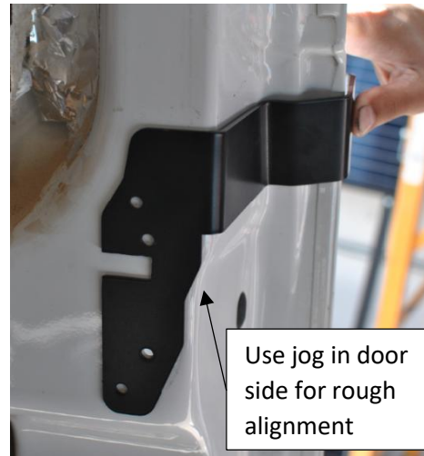
Figure 11: Dry Fit Bracket Up to Door
