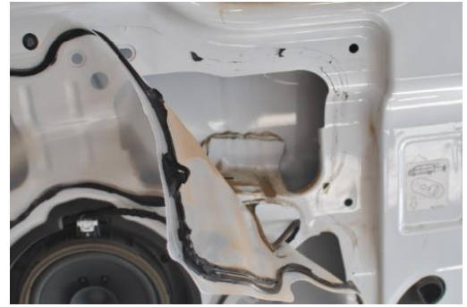
Figure 10: Inner Door Liner Peeled Back for Access
