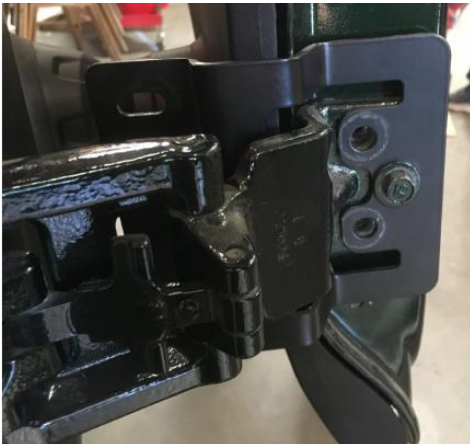
Figure 4: Hinge Placed Back into Position
