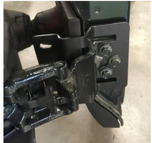
Figure 6: Inside View of Installed Lower Hinge Bracket
