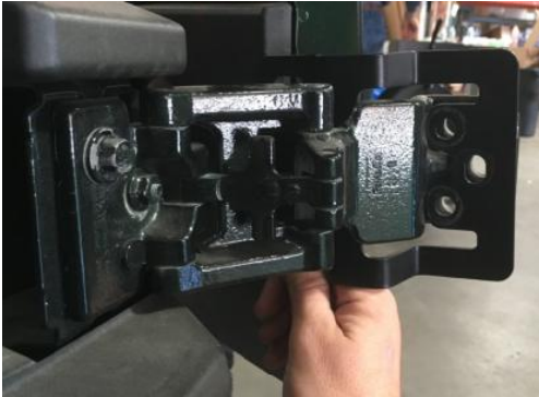
Figure 3: Bracket Installed Over Factory Hinge
