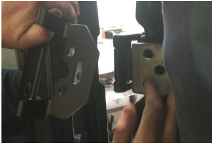
Figure 2: Upper Hinge Rotated Away from Door
