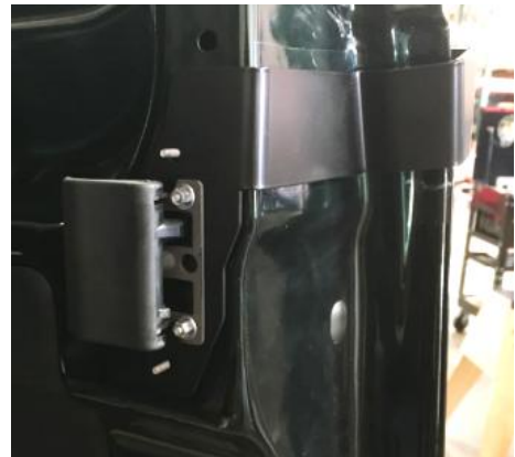
Figure 15: Upper Inner Passenger's Side Bracket Installed
