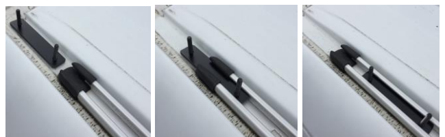
Figure 13: Track Threaded Insert Installation
