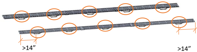
Figure 3: Mounting Bracket Locations
