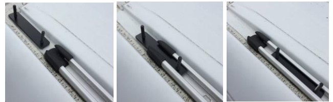
Figure 13: Track Threaded Insert Installation
