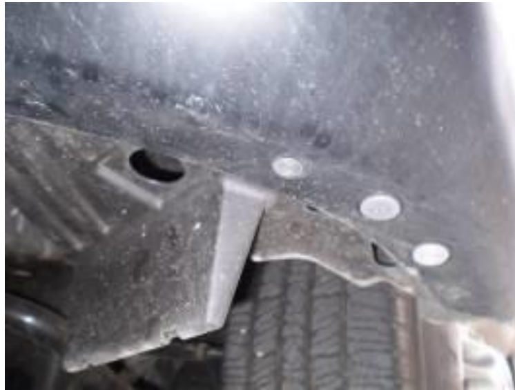
Figure 1. Remove 7 screws attaching the inner plastic fender.
