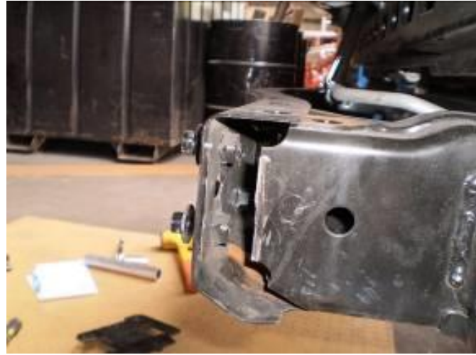
Figure 8b. Crossmember weld after cutting.
