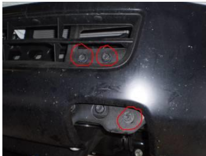
Figure 5. View from the front of the vehicle, 4 more bolts on the main bumper structure.
