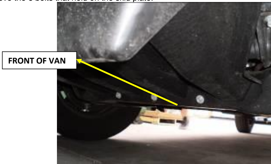
Figure 3. 6 bolts attaching the skid plate.
