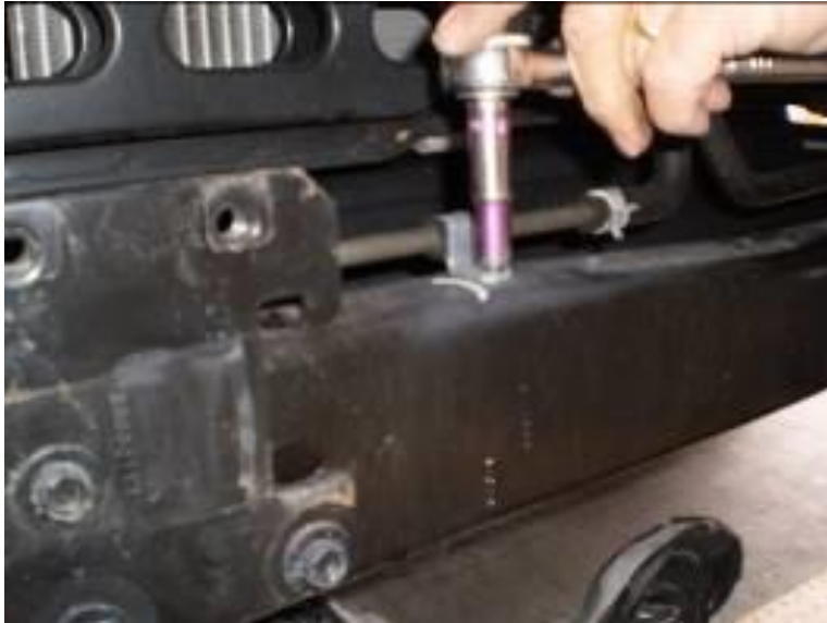
Figure 6. Bolts attaching cooler lines to the front crossmember.
