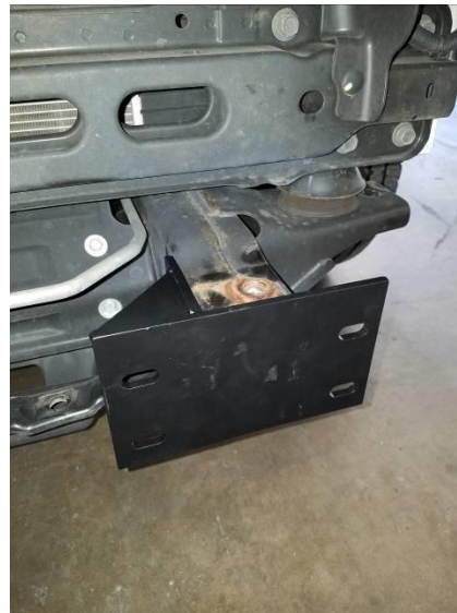
Figure 9. Steel angle brackets bolted to the passenger (left) and driver (right) frame horns.
