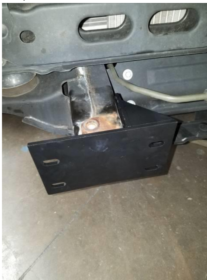
Figure 9. Steel angle brackets bolted to the passenger (left) and driver (right) frame horns.
