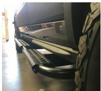
Figure 4: Alignment of Nerf Bar to Body Side
