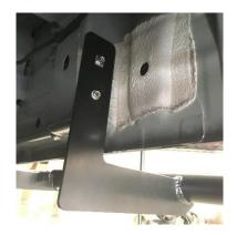
Figure 5: Rear Blade Secured into Position
