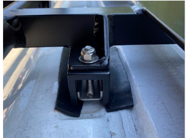
Figure 1: Promaster Roof Rack Mounting Installation
