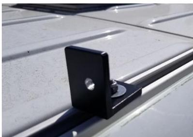
Figure 1: "L" Brackets Installed on Factory/Aftermarket Tracks
