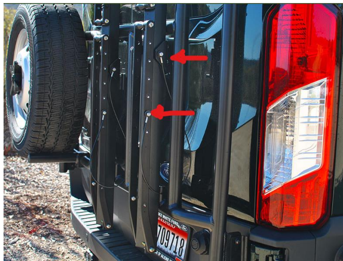
Figure 8: Steel Cable Location
