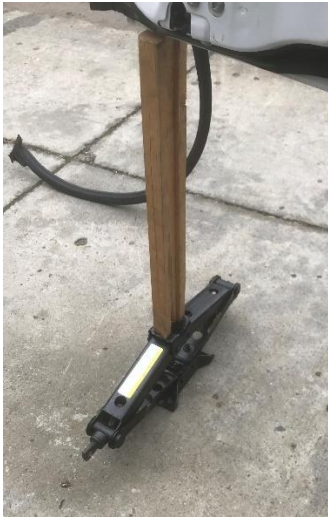
Figure 2: Support Door Prior to Installation
