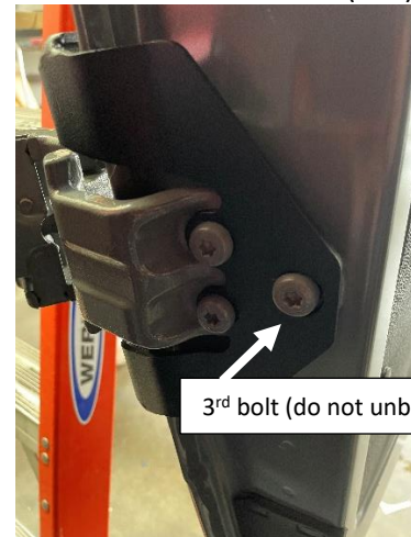
Figure 9: Bracket Installed Over Factory Hinge
