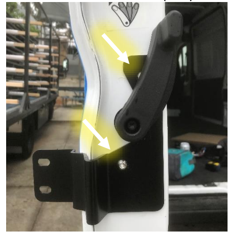
Figure 13: Inner Driver Door Bracket Installed
