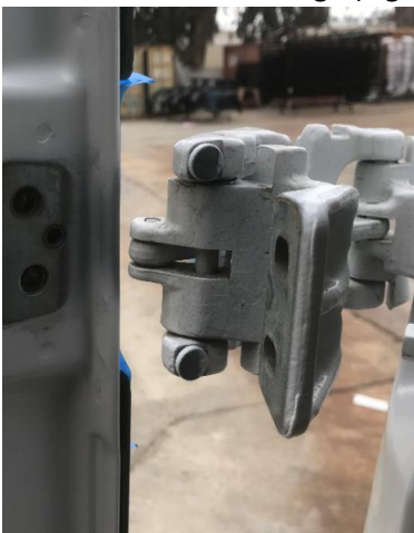
Figure 4: Upper Hinge Rotated Away from Door
