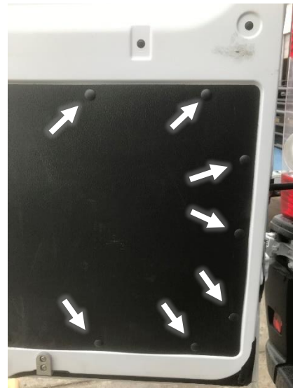
Figure 20: Remove Plastic Door Rivets
