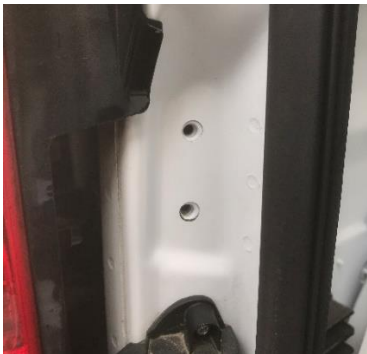
Figure 18: Factory Threaded Holes
