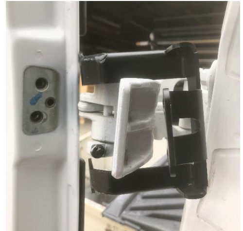
Figure 5: Bracket Installed Over Factory Hinge
