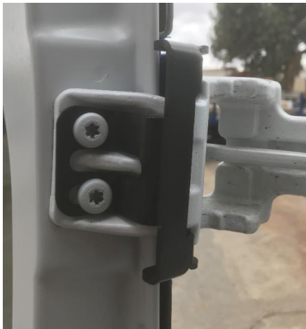
Figure 7: Inside View of Installed Upper Hinge Bracket
