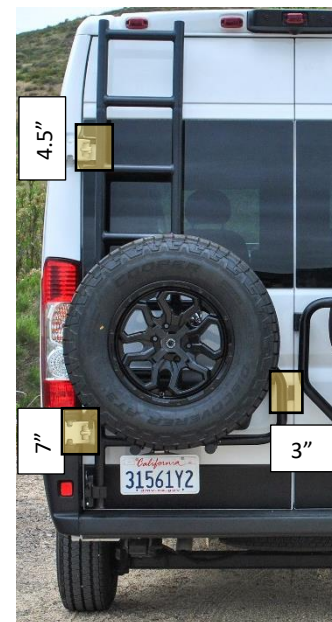
Figure 1: Locations of Protective Film Application
