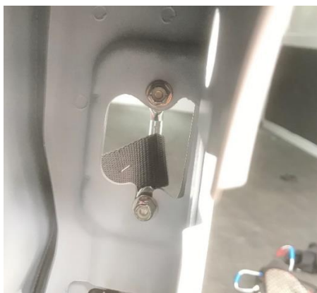
Figure 22: Backside View of Door Stop Mounting
