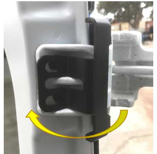
Figure 6: Bracket Installed Over Factory Hinge
