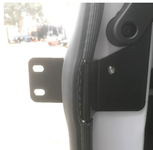
Figure 16: Installed Weather Stripping After Modification
