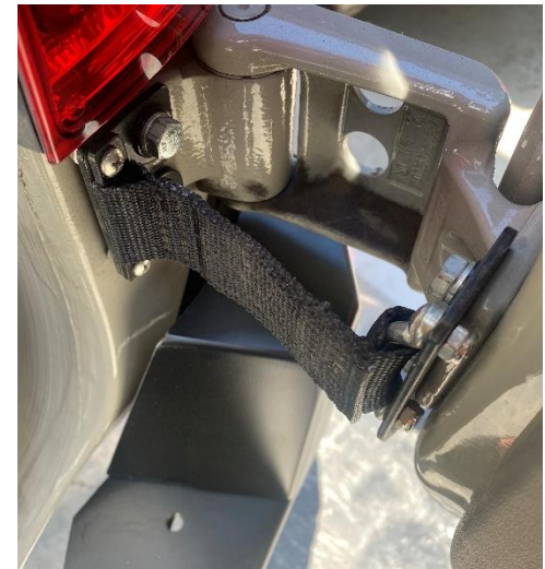
Figure 10: Limiting Strap Installed
