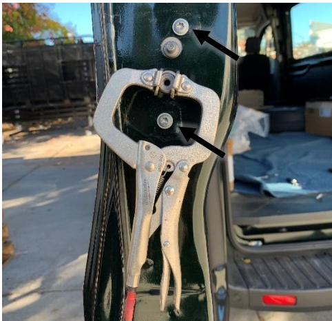
Figure 7: Inner Door Bracket Installed
