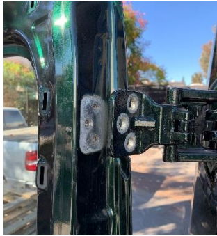
Figure 2: Upper Hinge Rotated Away from Door
