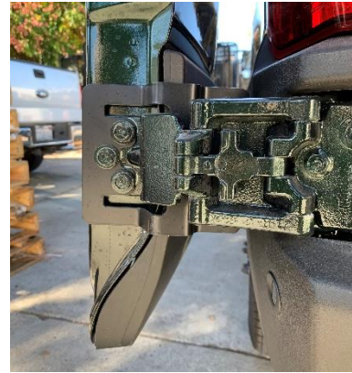
Figure 5: Inside View of Installed Lower Hinge Bracket
