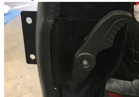
Figure 12: Installed Weather Stripping After Modification
