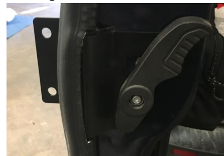
Figure 12: Installed Weather Stripping After Modification
