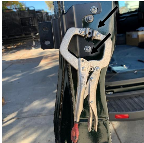
Figure 8 Inner Driver Door Bracket Installed
