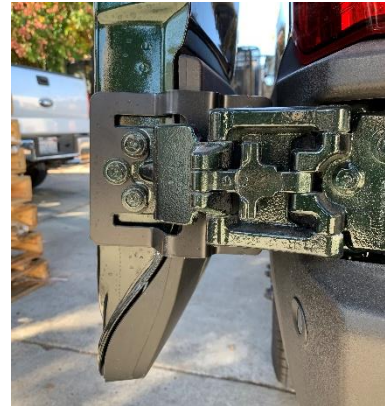
Figure 5: Inside View of Installed Lower Hinge Bracket
