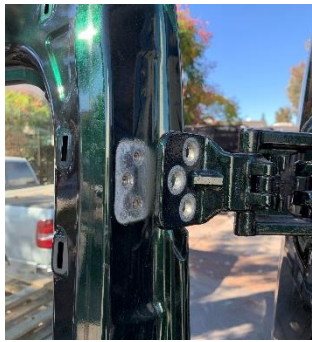
Figure 2: Upper Hinge Rotated Away from Door
