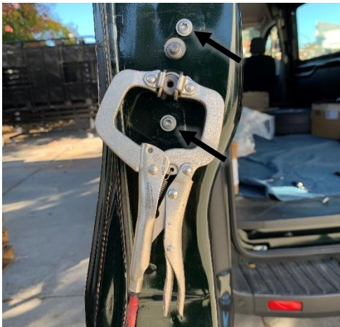
Figure 7: Removing Factory Torx Screws
