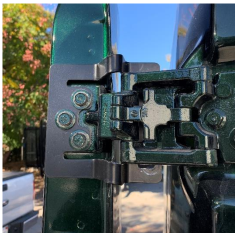
Figure 4: Inside View of Installed Upper Hinge Bracket
