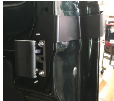
Figure 15: Upper Inner Passenger's Side Bracket Installed
