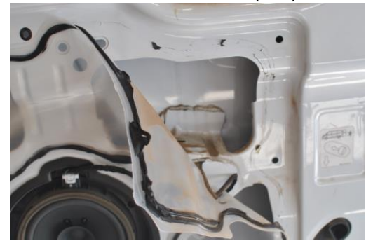
Figure 10: Inner Door Liner Peeled Back for Access
