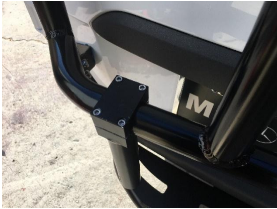
Figure 7: Bolt-On Supports Loosely Bolted to Lower Crossmember
