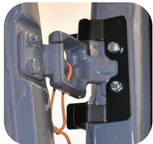
Figure 9: Upper Bracket, Installed Upper Bolt
