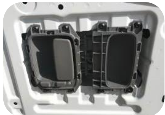
Figure 14: Inner Door Handle Removal
