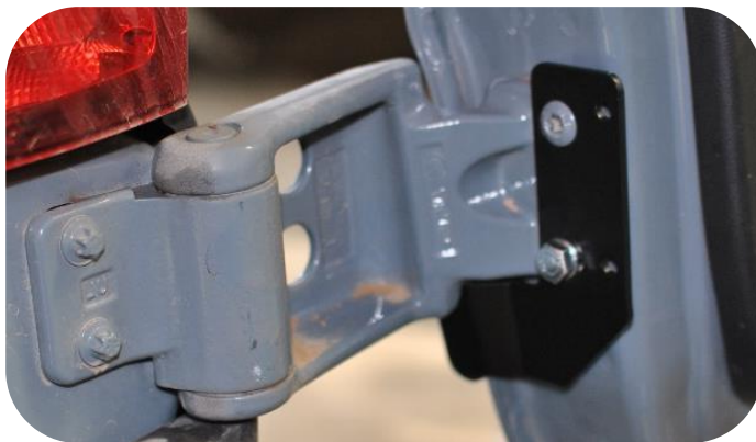
Figure 11: Lower Bracket, Installed Lower Bolt
