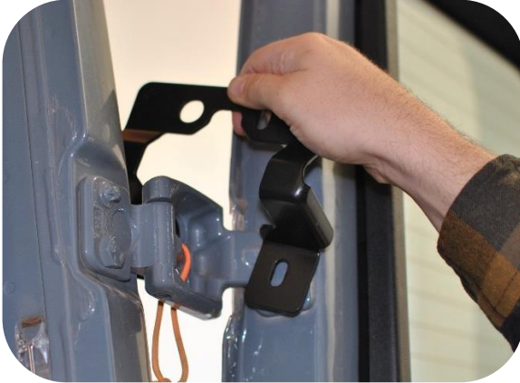
Figure 4: Fitting Upper Bracket over the Hinge
