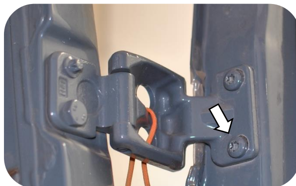
Figure 3: Upper Hinge, Bolt to Remove
