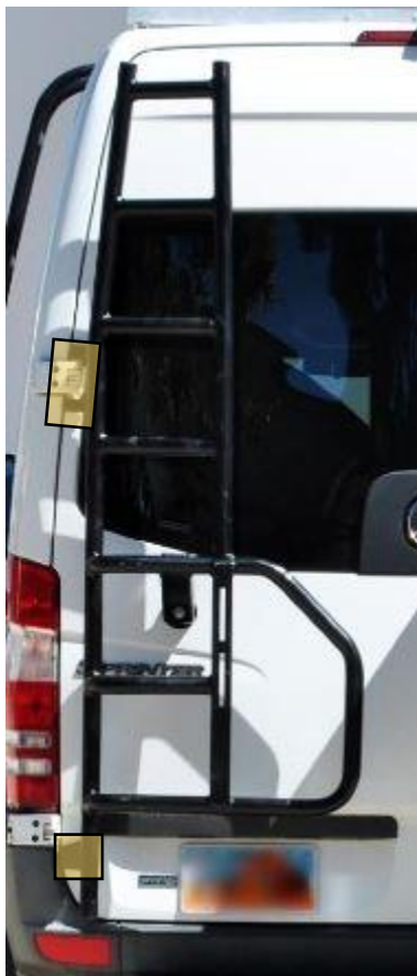
Figure 1: Protective Tape Locations on Door
