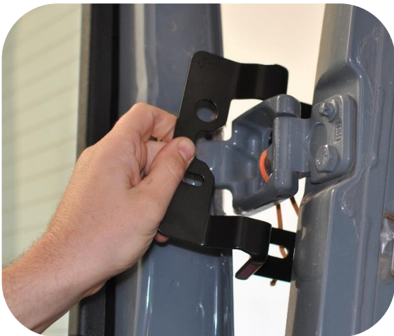
Figure 5: Rotating Upper Bracket into Position
