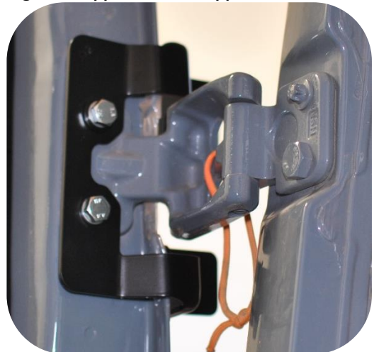
Figure 9: Upper Bracket, Installed Upper Bolt
