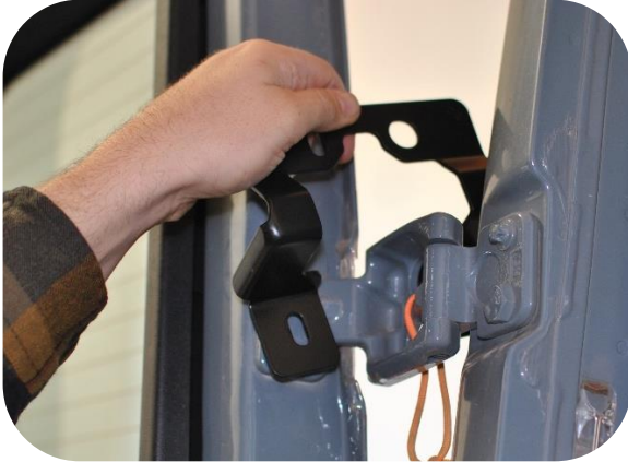
Figure 4: Fitting Upper Bracket over the Hinge
