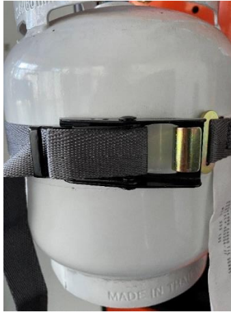
Figure 5: Propane Tank Secured with Latch and Hook
