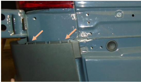
Figure 8: Small Plastic Panel Removed
