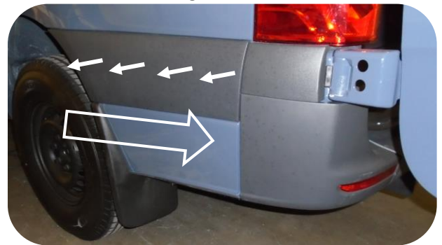
Figure 5: Side Panel Removal
