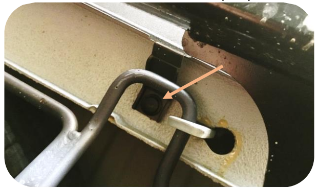
Figure 3: Plastic Rivets Underneath Bumper
