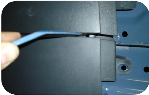
Figure 7: Removing Small Plastic Panel from Rear Bumper
