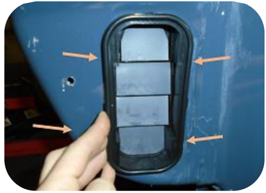
Figure 9: Removal of Air Pressure Relief Insert
