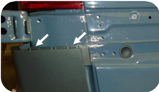
Figure 8: Small Plastic Panel Removed
