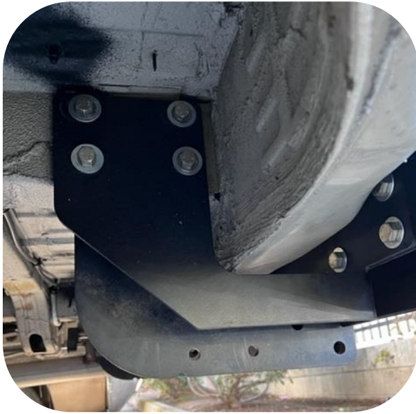
Figure 11: Bumper Mounted on Frame
