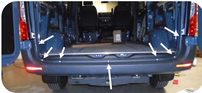
Figure 2: Torx Bolts on the Rear Bumper
