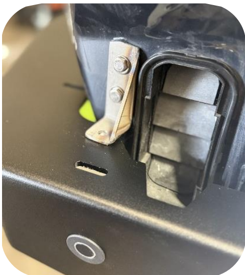
Figure 13: Installed Air Pressure Relief Insert
