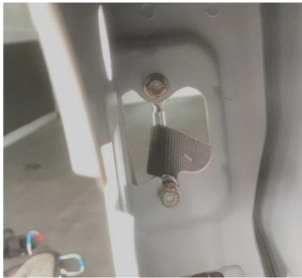
Figure 13: Backside View of Door Stop Mounting
