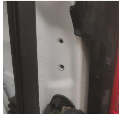
Figure 15: Factory Threaded Holes on Inside of Door Jam
