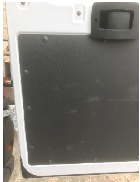
Figure 11: Remove Plastic Door Rivets
