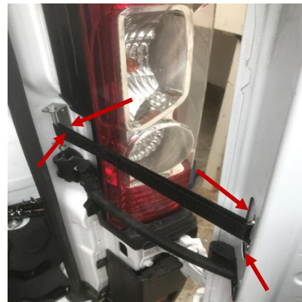
Figure 18: Completed Door Strap Installation
