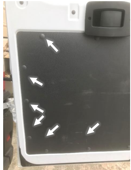
Figure 12: Remove Plastic Door Rivets
