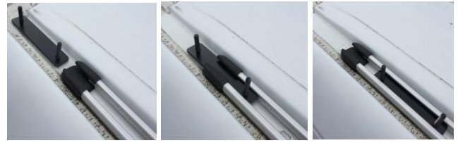
Figure 14: Track Threaded Insert Installation
