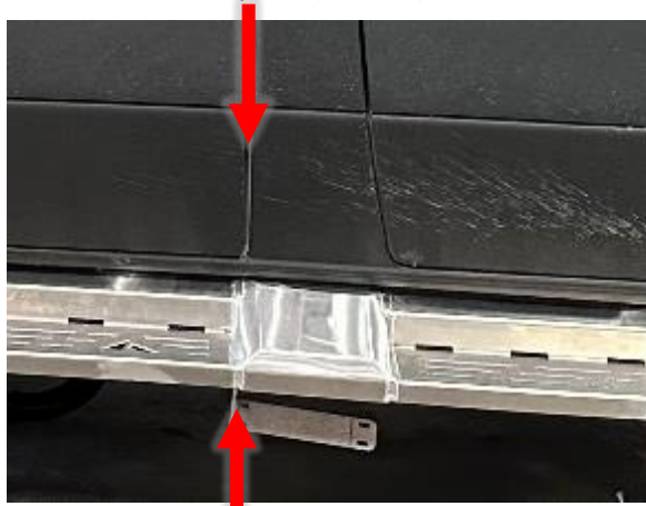
Figure 1: Side Step Alignment with B-Pillar Seam
