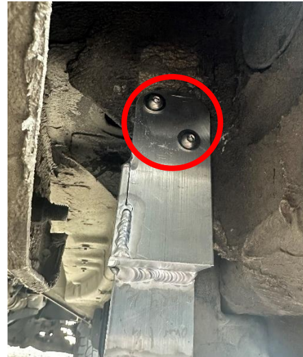
Figure 7: Rear Support Bracket Upper Mounting
