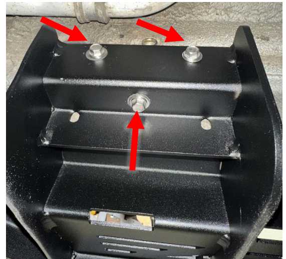
Figure 2: Step Bracket Installation Behind Pinch Weld
