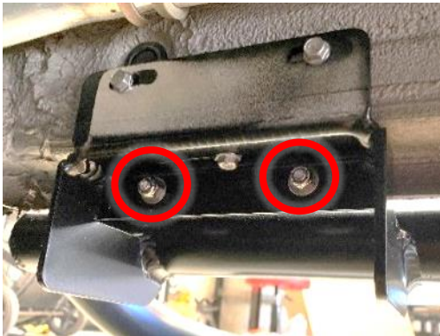
Figure 5: Pinch Weld Fastener Installation
