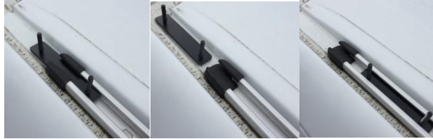
Figure 1: Threaded inserts installed onto tracks
