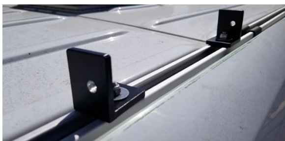
Figure 1: "L" Brackets Installed on Factory/Aftermarket Tracks
