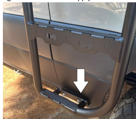
Figure 4: Lower Bracket Tightening Technique.
