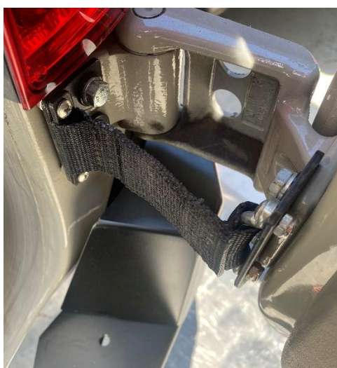
Figure 13: Limiting Strap Installed
