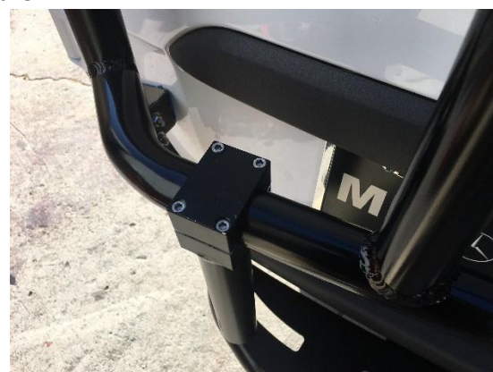
Figure 14: Bolt-On Supports Loosely Bolted to Lower Crossmember
