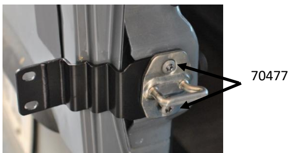
Figure 5: Driver's Inside Door Latch Bracket Installed
