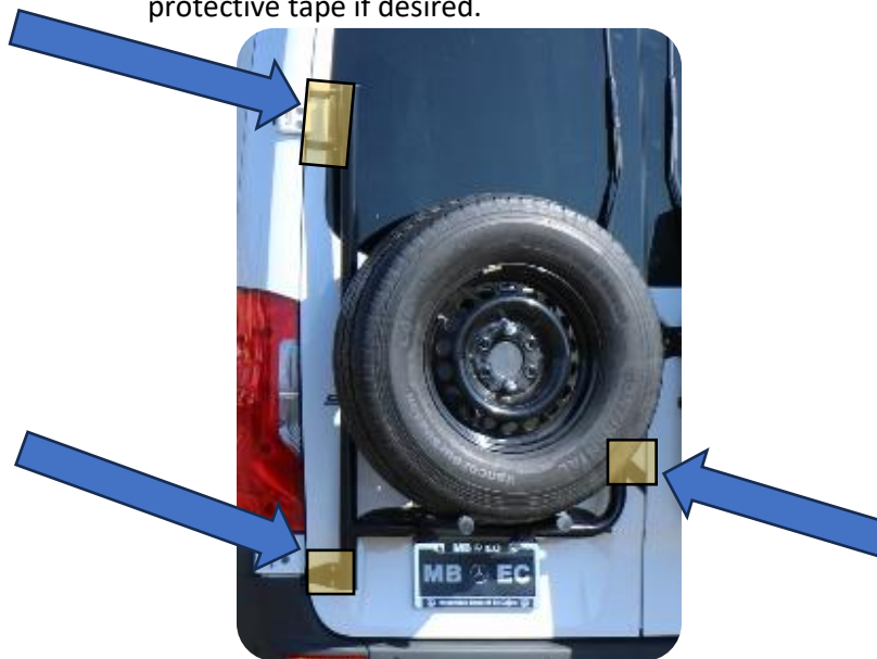
Figure 3: Protective Tape Locations on Door
