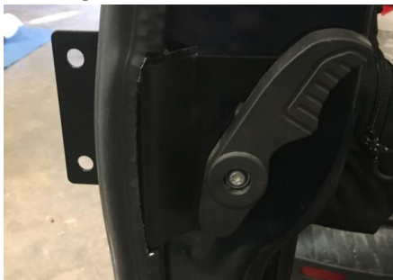
Figure 12: Installed Weather Stripping After Modification
