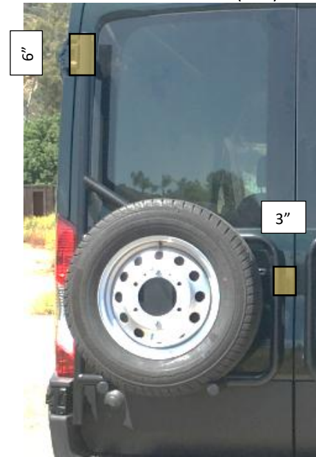
Figure 1: Locations of Protective Film Application
