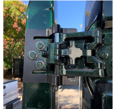
Figure 4: Inside View of Installed Upper Hinge Bracket
