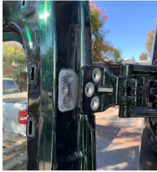
Figure 2: Upper Hinge Rotated Away from Door
