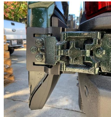
Figure 5: Inside View of Installed Lower Hinge Bracket
