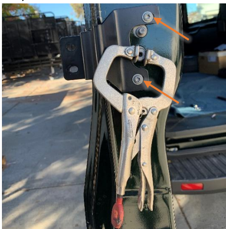
Figure 8: Inner Driver Door Bracket Installed
