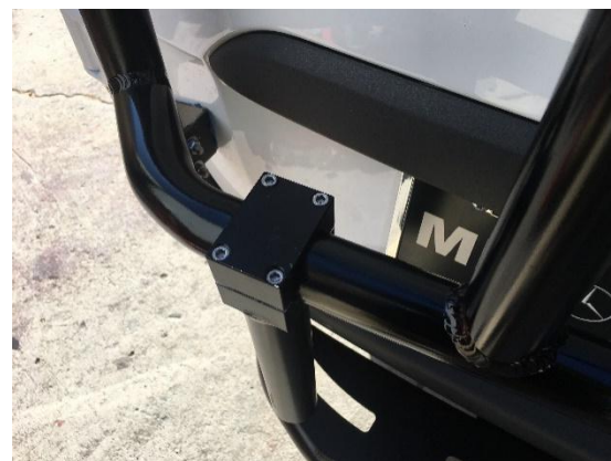
Figure 4: Bolt-On Supports Loosely Bolted to Lower Crossmember
