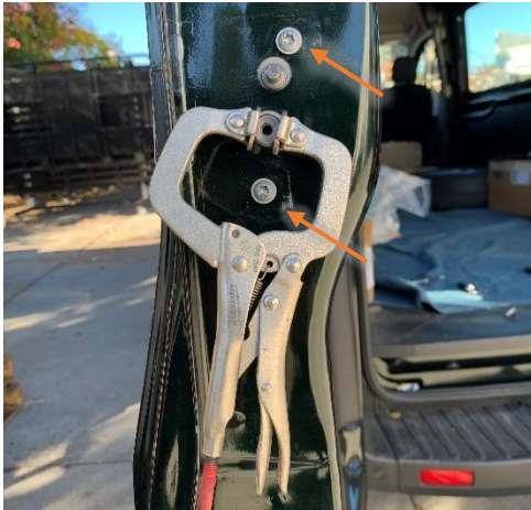
Figure 7: Removing factory torx screws
