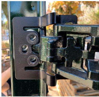
Figure 3: Bracket Installed Over Factory Hinge
