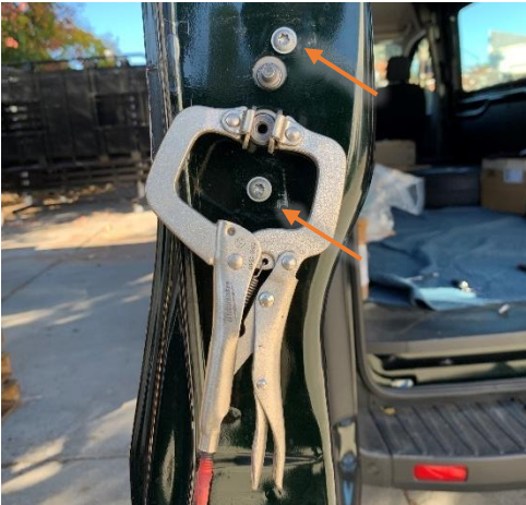
Figure 7: Removing factory torx screws
