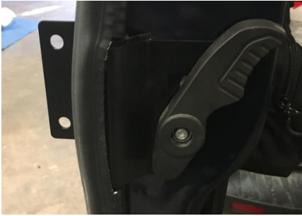
Figure 12: Installed Weather Stripping After Modification
