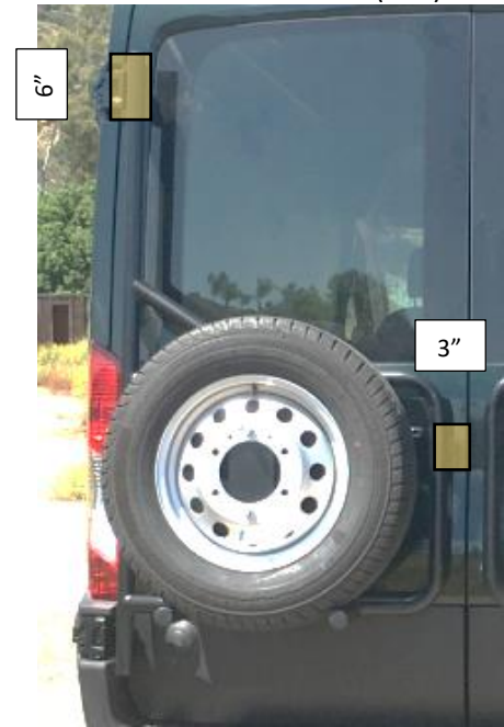
Figure 1: Locations of Protective Film Application
