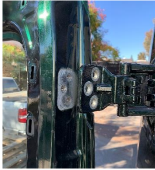
Figure 2: Upper Hinge Rotated Away from Door
