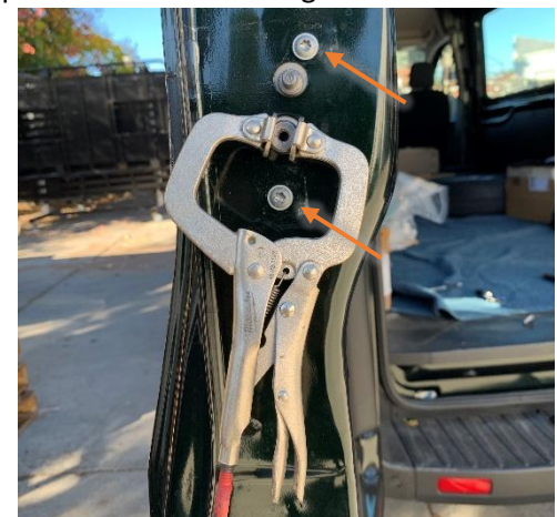
Figure 7: Removing Factory Torx Screws
