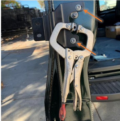
Figure 8: Inner Driver Door Bracket Installed
