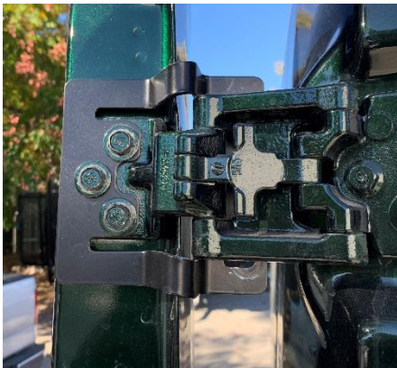
Figure 4: Inside View of Installed Upper Hinge Bracket
