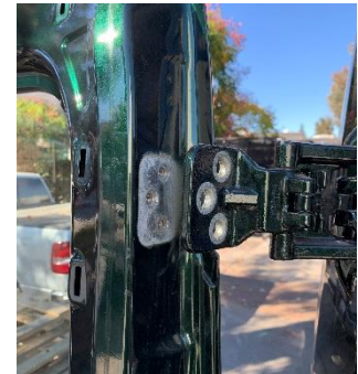
Figure 2: Upper Hinge Rotated Away from Door
