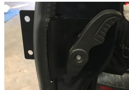
Figure 12: Installed Weather Stripping After Modification
