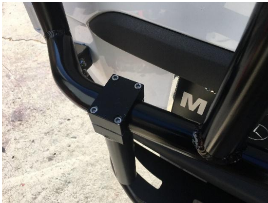
Figure 4: Bolt-On Supports Loosely Bolted to Lower Crossmember
