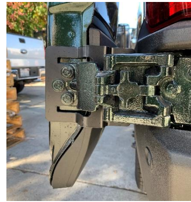
Figure 5: Inside View of Installed Lower Hinge Bracket
