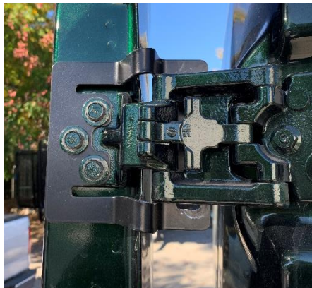
Figure 4: Inside View of Installed Upper Hinge Bracket
