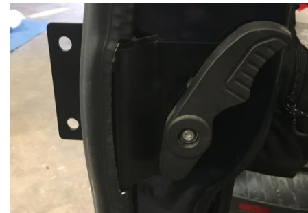
Figure 12: Installed Weather Stripping After Modification
