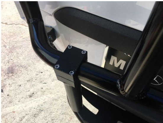
Figure 4: Bolt-On Supports Loosely Bolted to Lower Crossmember
