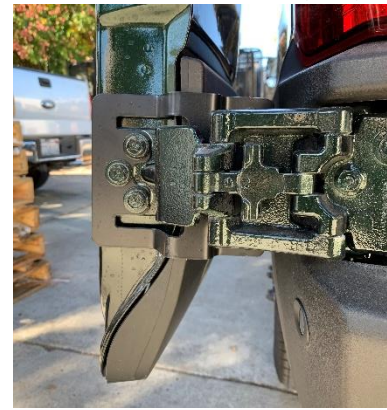
Figure 5: Inside View of Installed Lower Hinge Bracket
