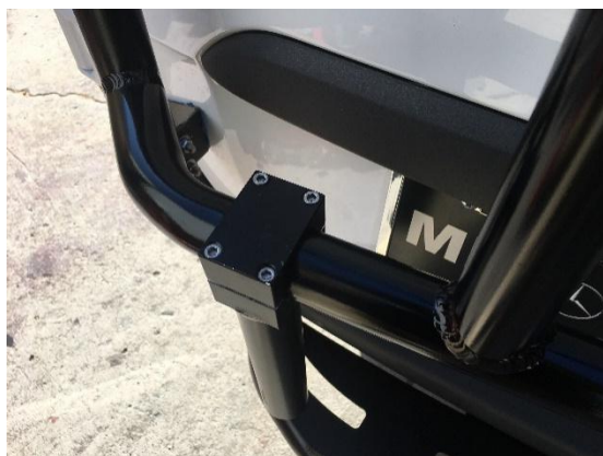
Figure 1: Bolt-On Supports Loosely Bolted to Lower Crossmember
