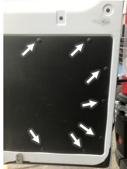
Figure 19: Remove Plastic Door Fasteners
