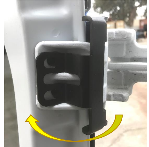
Figure 6: Bracket Installed Over Factory Hinge
