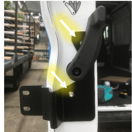
Figure 12: Inner Driver Door Bracket Installed
