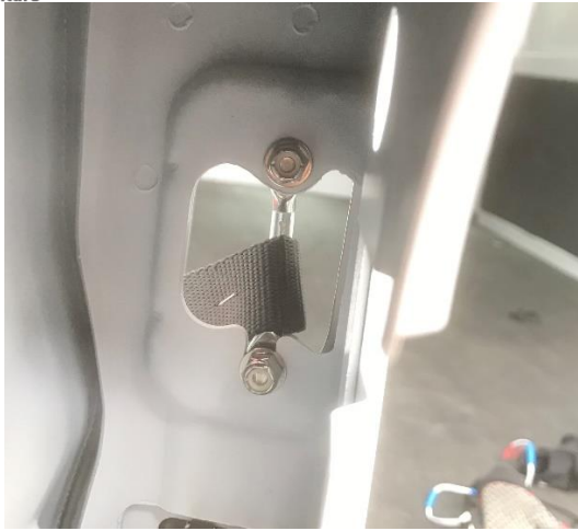
Figure 21: Backside View of Door Stop Mounting
