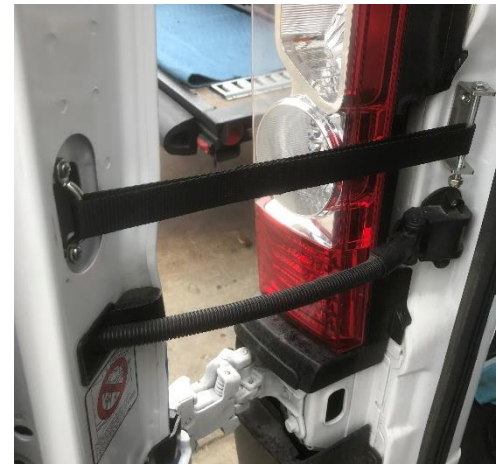
Figure 24: Complete Door Stop Install
