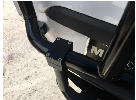
Figure 1: Bolt-On Supports Loosely Bolted to Lower Crossmember
