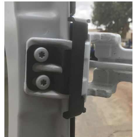
Figure 7: Inside View of Installed Upper Hinge Bracket
