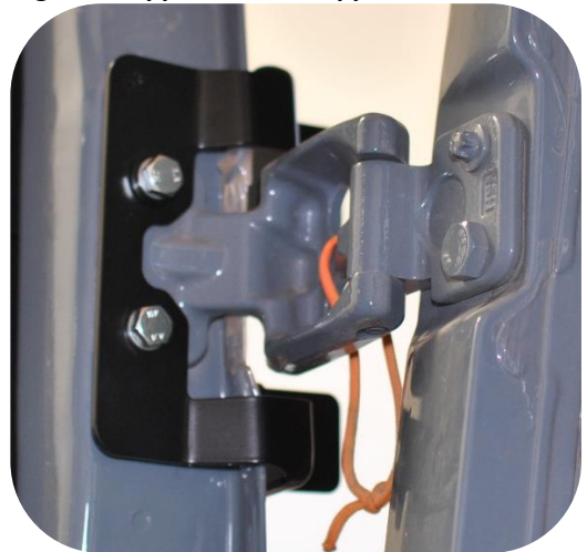
Figure 9: Upper Bracket, Installed Upper Bolt
