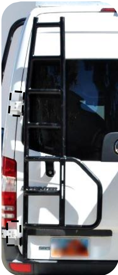
Figure 2: Protective Tape Vehicle Locations
