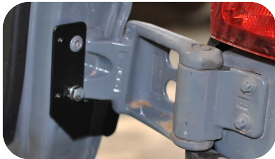
Figure 11: Lower Bracket, Installed Lower Bolt
