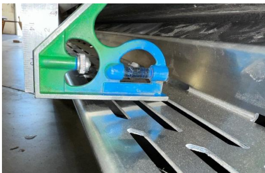
Figure 5: Verification that the Step is Level
