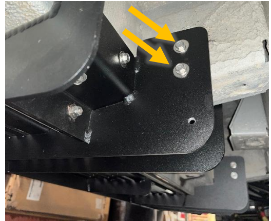
Figure 7: Unibody Self-Tapping Screw Example
