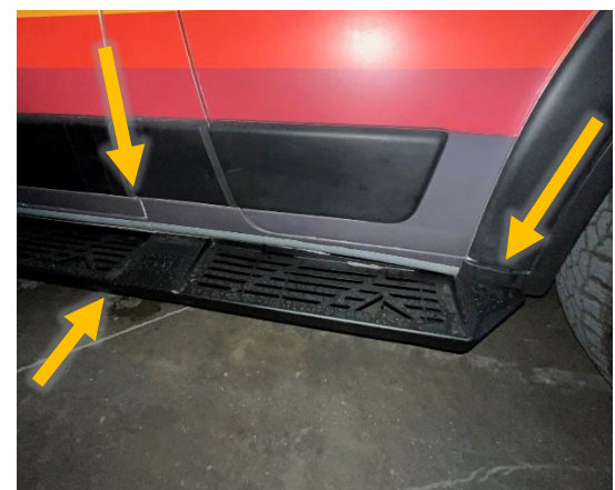
Figure 3: Side Step Alignment with B-Pillar Seam and Front Fender Flare
