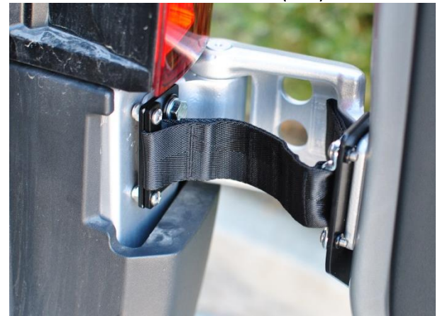
Figure 8: Door Limiting Strap Installed
