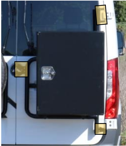
Figure 1: Protective Tape Locations on Door
